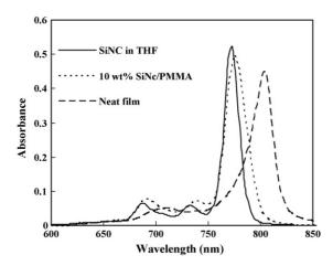
Fig. 2. Absorption spectra of the SiNc in THF solution (solid line), a 10 wt% SiNc/PMMA film (dotted line) and a neat SiNc film (broke line).
