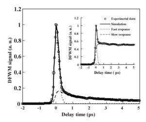
Fig. 4. Simulation for a temporal profile of DFWM signal of a neat SiNc film by assuming Förster type energy transfer, open circles, solid line, dotted line and broke line represent experimental data, simulation, fast component and slow component, respectively. Inset: a simulation for a temporal profile of DFWM signal of SiNc in THF solution by a biexponential function.
