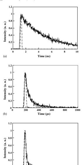
Fig. 5. Fluorescence decay curves of SiNc in different media. (a) SiNc in THF solution; (b) a 10 wt% SiNc/PMMA film; (c) a neat SiNc film. Excitation wavelength was 400 nm. Broken lines represent the response function to laser excitation pulse.
