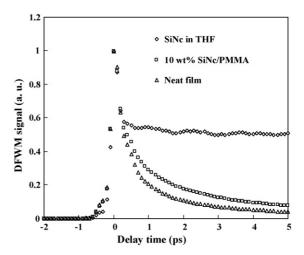
Fig. 3. Temporal profiles of DFWM signal of the SiNc in THF solution, a  $10~\rm wt\%$  SiNc/PMMA film and a neat SiNc film.
